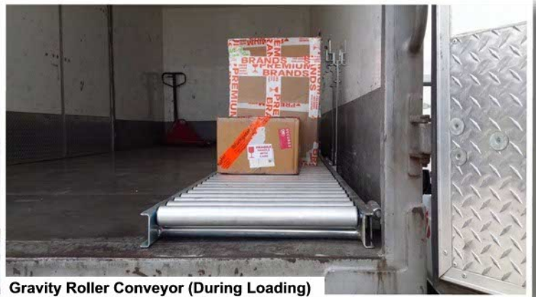
Gravity Roller Conveyor (During Loading)
